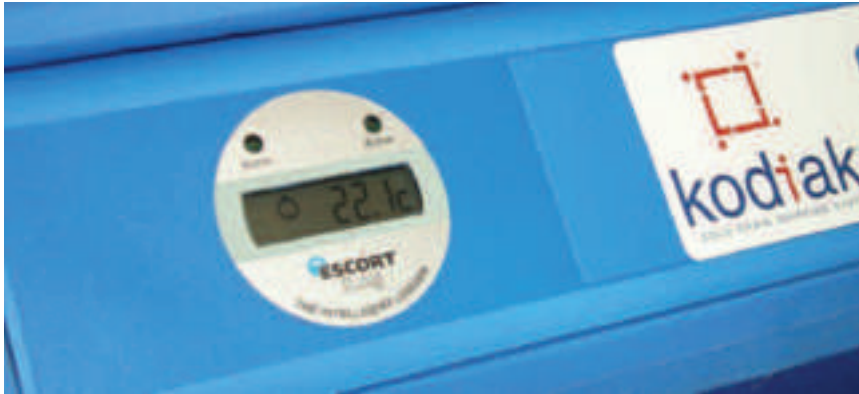
Escort loggers have a bookmark feature that places a mark at certain data points when a magnet is touched to the unit. This is handy to track when boxes go through sorting centers, distribution points, etc., says Don Pagel of Kodiak.
