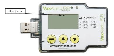
Press and hold the Start/Stop button for 3 seconds. The device will display the start delay screen as shown below (run icon (→) and start delay icon (▲) are displayed). The display will count down the programmed start delay time until 0 minutes remain. At the end of the start delay countdown, the start delay icon will turn off and the VaxAlert will enter measurement (run) mode.
