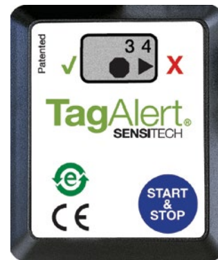
Holding Start & Stop button starts AlarmAlert mode, first displaying number of alarm, day of alarm, then timeframe alarm was triggered; This example shows alarm triggered day 7 of trip
