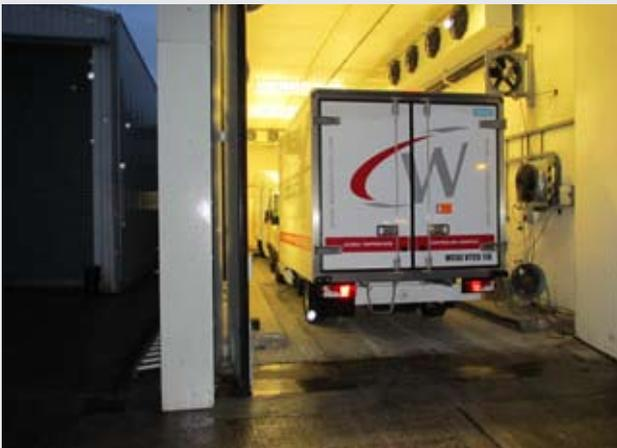
When creating the test protocol we decided to stress test at very high and very low temperatures which are at the limits of what we might expect to experience on the road. We set the high external temperature to +40°C, and the test chamber achieved between 38-40°C during the test. The lowest external was set at -25°C and the test chamber achieved between -22°C and -25°C.
