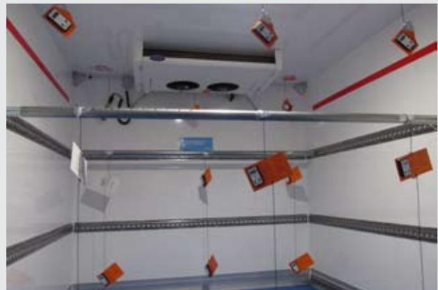
Pallets of the test substrate material were conditioned in a temperature controlled reefer positioned outside the CRT test facility, so that way it could be pre-conditioning for the next temperature requirement whilst the previous test was running. We added twenty seven Sensitech temperature monitors inside each vehicle, together with a further eight thermocouples from CRT. No change in temperature was going to go unrecorded!
