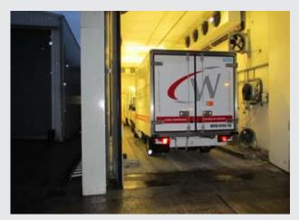
When creating the test protocol we decided to stress test at very high and very low temperatures which are at the limits of what we might expect to experience on the road. We set the high external temperature to  $+40^{\circ}$ C, and the test chamber achieved between 38-40°C during the test. The lowest external was set at -25°C and the test chamber achieved between  $-22^{\circ}$ C and  $-25^{\circ}$ C.
