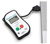
**Note:** Do not remove the plug from the USB port on the computer until the LED on the face of the unit glows solid **GREEN**.
