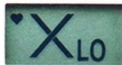
Low alarm activated
