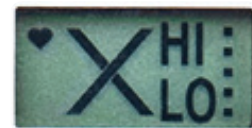
High and low alarm activated
